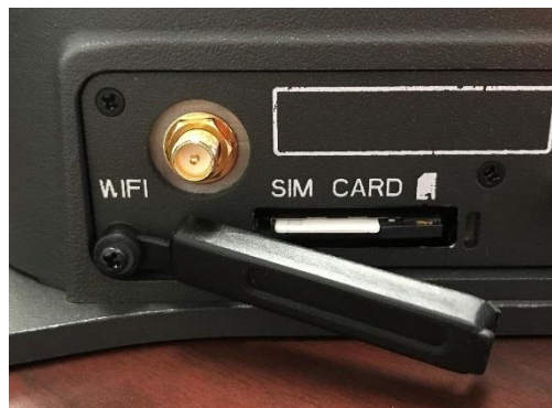
Figure 2-8 SIM Card with Cover Opened
