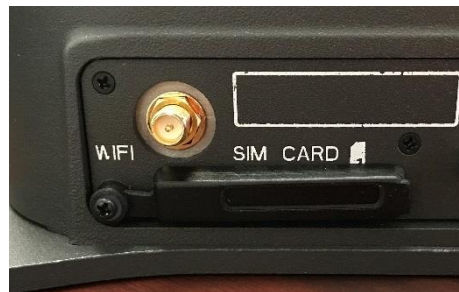
Figure 2-10 Secure the SIM Card Cover
