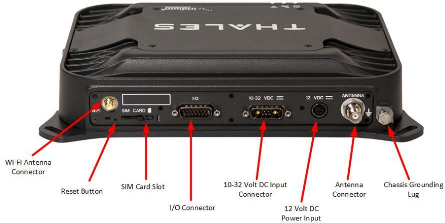
Figure 1-5 Terminal Unit (TU) Back Panel Detail
